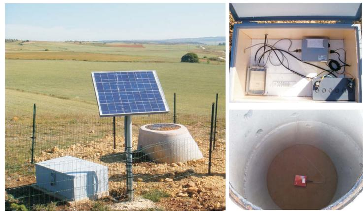
Image of the installation of one seismic station at the field.
